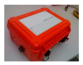
The eentec DR4050 is a *rugged*, *ultra low power*, *high-performance*, *versatile 24-bit and 21-bit resolution seismic recorder*. It is designed for the most demanding requirements in high performance seismic or strong motion research. Generally for structural monitoring and other seismic applications, only the 21-bit (low resolution 24-bit ADC) is required. The standard unit has an external sensor input.
